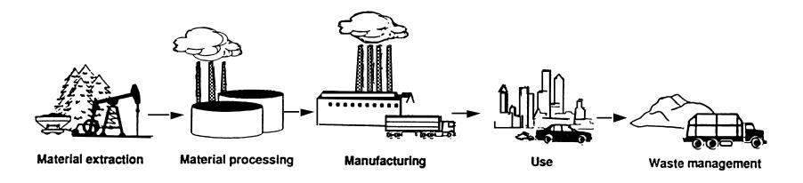
A paradigm that provides a holistic picture of an entire product system covering resources extraction, material processing, transportation, manufacturing, distribution, use, disposal and reuse/recycling.
