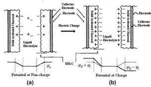
EDLCs are also known as Ultracapacitors or Supercapacitors have very high capacitances.
