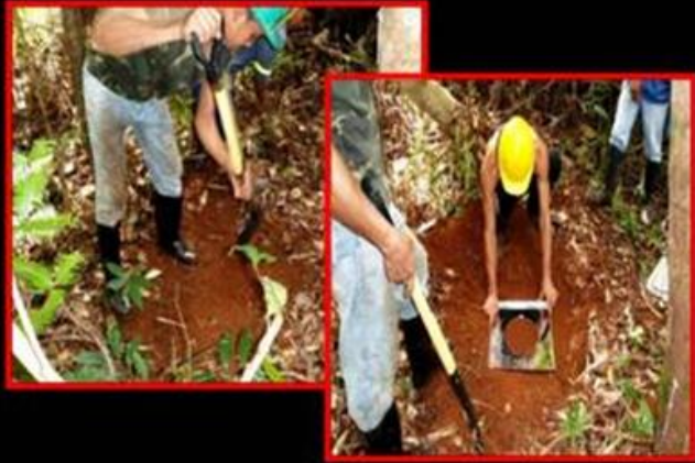
Ground clearing and template set up
