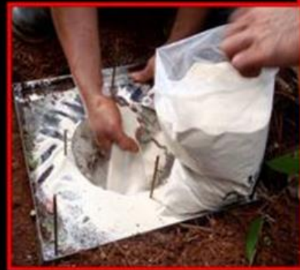
Retrieval of excess sand from apparatus and sand in cone and mold
