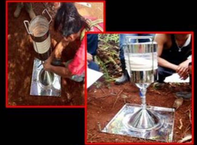
Apparatus set up and volume of sand in mold determination
