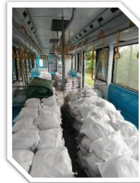
Sand Loading for Design Load and Crush Load
