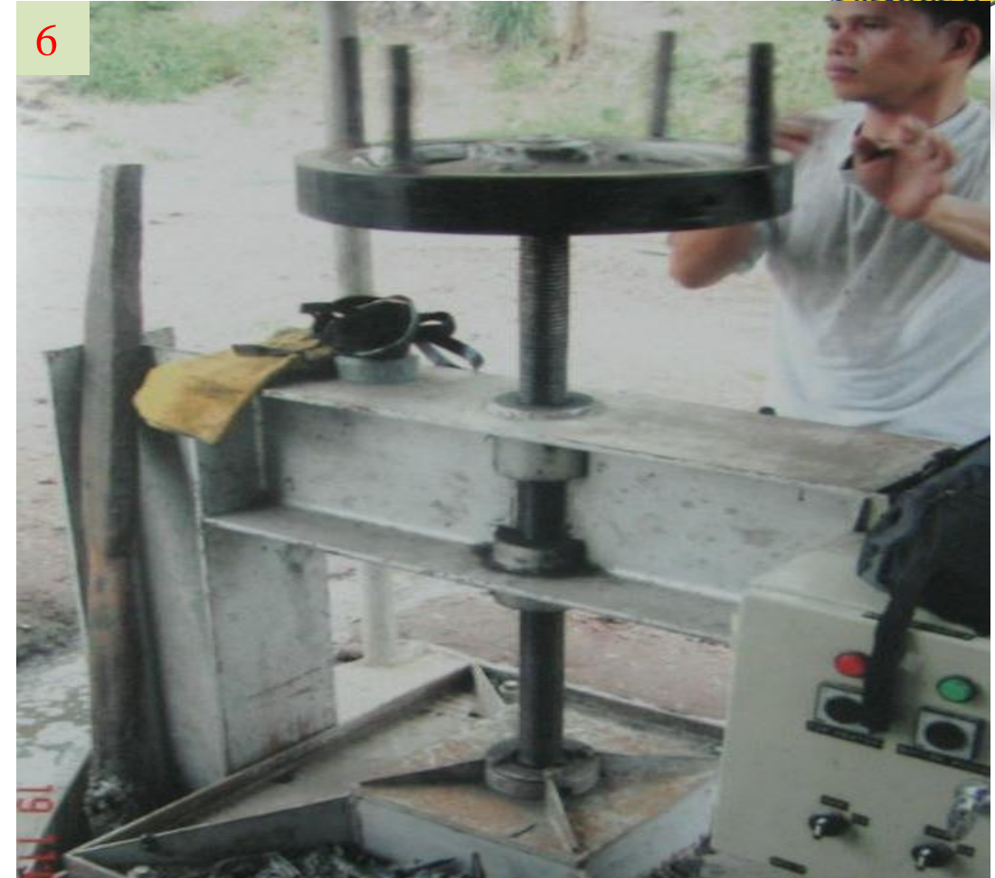
Cold-pressing the formed material to certain thickness using the screw-type fabricated press
