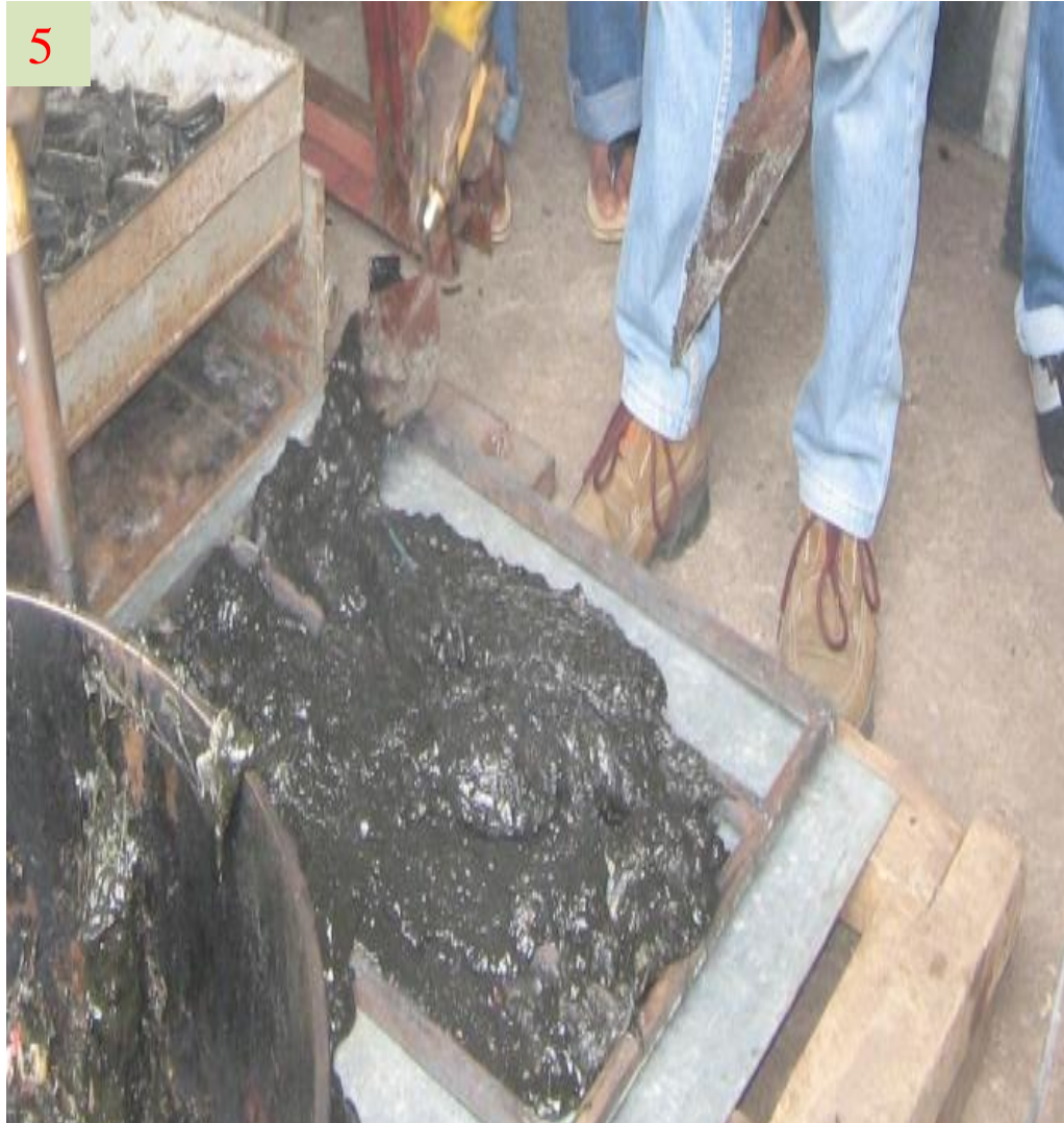
Forming the mix materials in fabricated moulds
