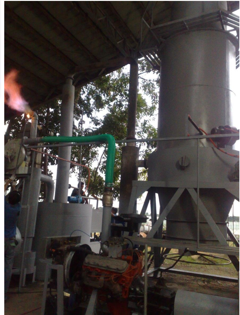
Rice hull gasifier for 100 kW electric power generation
