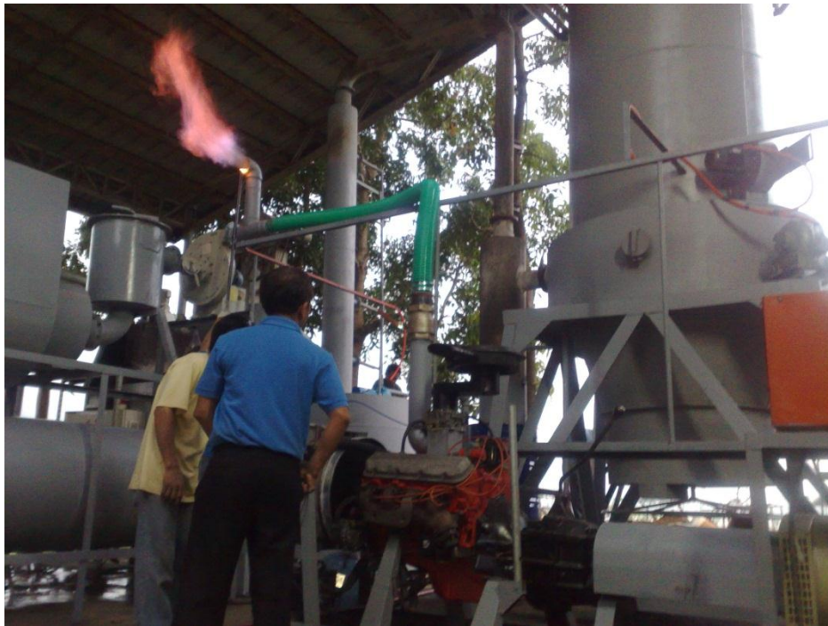
Rice hull gasifier for 100 kW electric power generation
